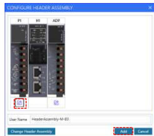
7. Added Header assembly is displayed in tree view as well as in System tab of working area as beside.
